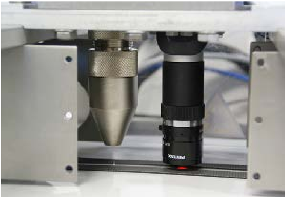
The camera checks every micro-perforation according to diameter and shape.
