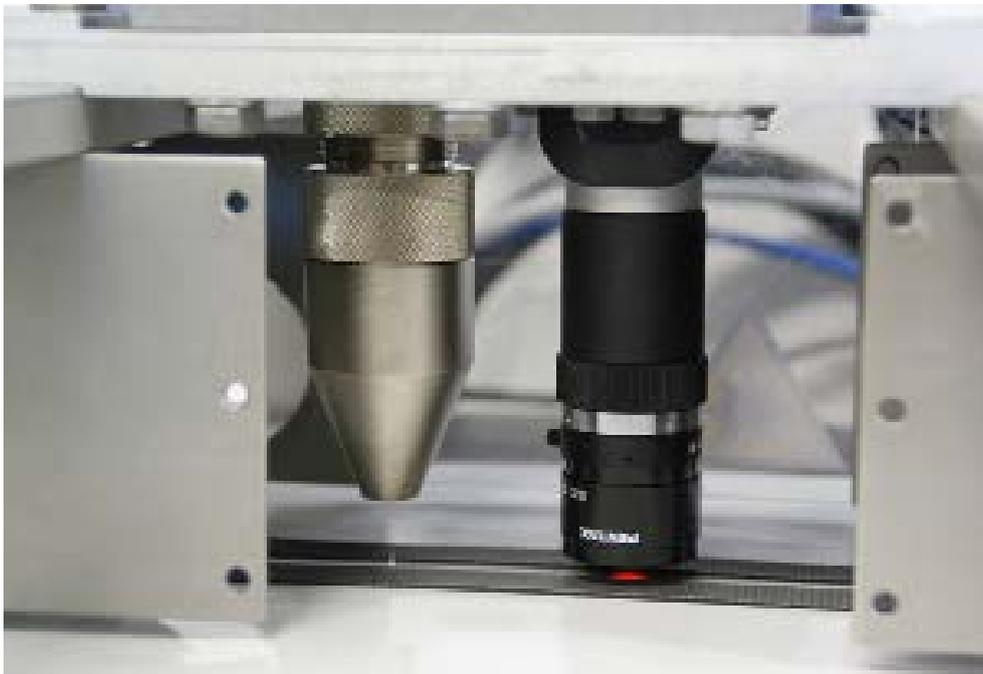
The camera checks every micro-perforation according to diameter and shape.
